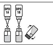
Immediately insert tube into chamber. Close lid. Select **Scan Sample**. Record result as Free Chlorine.
