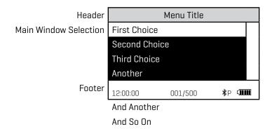
A light bar will indicate the menu choice. As the menu is scrolled through, the light bar will highlight different menu choices. Pressing the button will select the menu choice that is indicated by the light bar.
