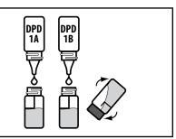
Immediately insert tube into chamber. Close lid. Select Scan Sample. Record result as Bromine.
