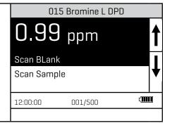
NOTE: For the most accurate results, samples over 7 ppm bromine should be diluted with chlorine demand free water and re-tested.
