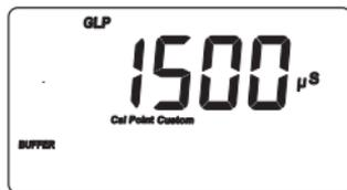
If the cell constant was changed after calibration (through the “CELL” setup function), this information is not displayed.
