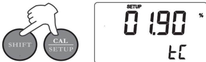
Select the desired setup item using the arrow keys, then press CFM to select and edit the setup item value, and its current value starts blinking (if it is a changeable parameter).
