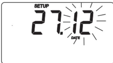
Press the arrow keys to change the value and CFM to confirm.
