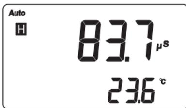
Press the HOLD key again to return to normal measurement mode.
